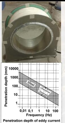
AC Degaussing: Pass the part slowly through the coil. Each magnetic domain will experience a gradually reducing and reversing field as it moves away from the center of the coil.
