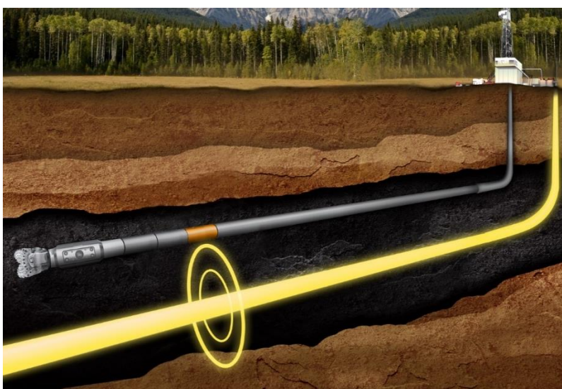
Figure 14—SA-AMR uses well-head access to induce a magnetic field in the target well (shown in yellow above) which is then utilized by a downhole sensor in the drilling BHA
