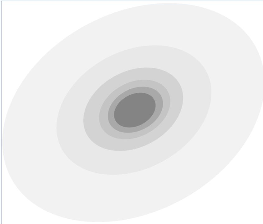
The Probability Density of the relative wellbore positions is illustrated by the concentric ellipses/ellipsoids.
