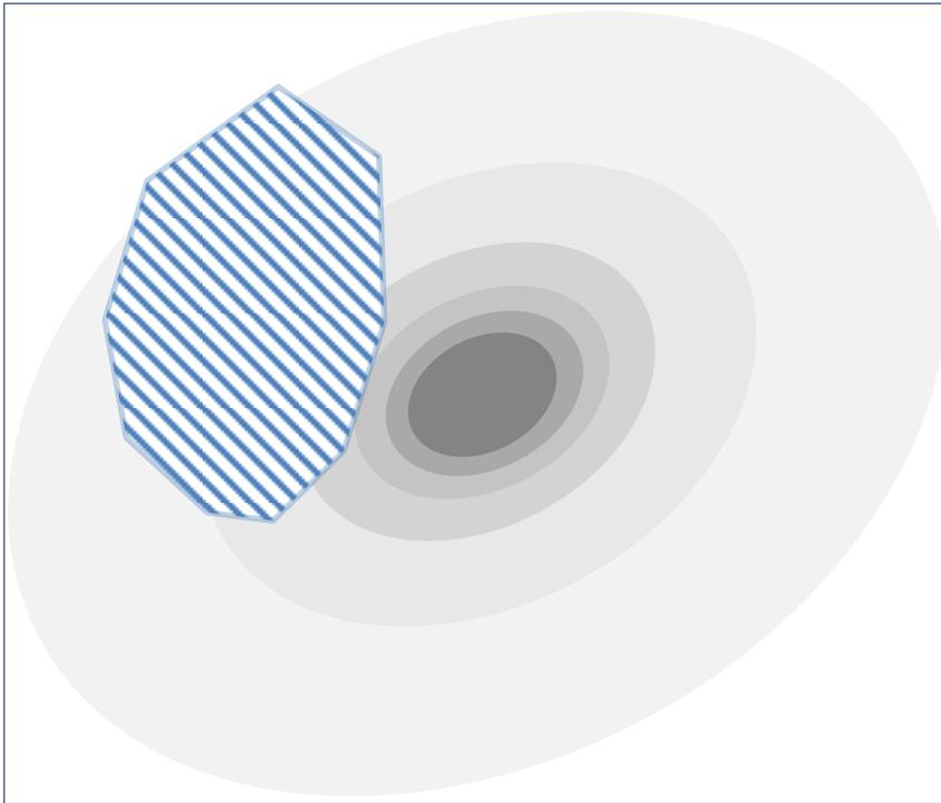
The Collision Probability is the probability density integrated over the appropriate area/ volume of the probability density.
