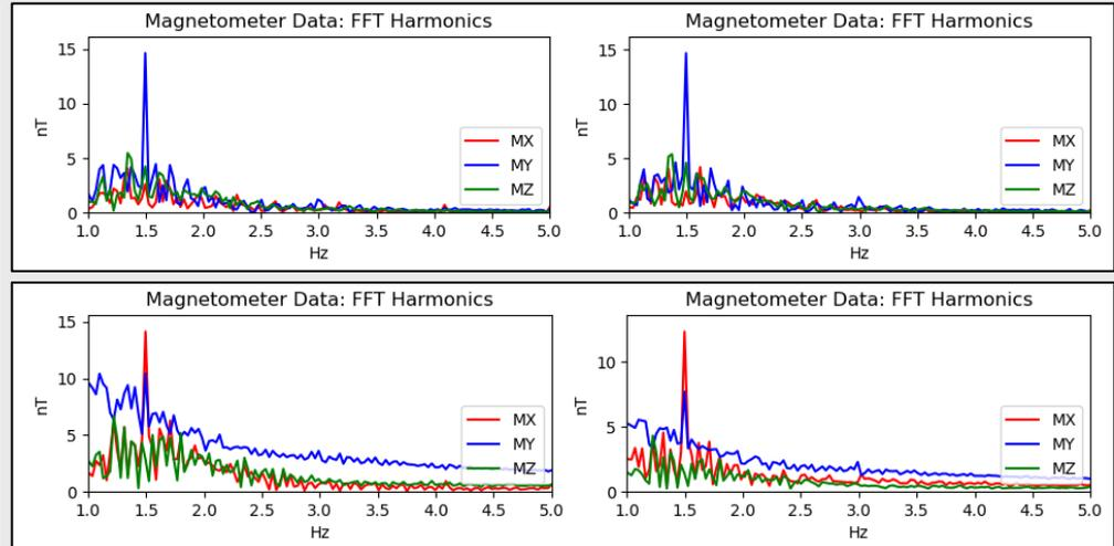
\*Readings from the AMR-WD gradient probe are shown in pairs to illustrate sensor array data
