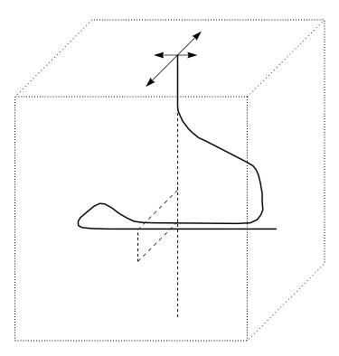
The well starts vertical, builds and drops to the East, returns back underneath the wellhead, builds above horizontal, then turns through 180° and finishes horizontal due East.
