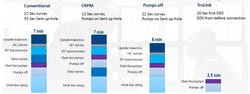
Comparison of MWD survey time between diverse acquisition methods (Courtesy of SLB)
