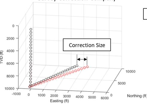
Step 6: Calculate Error in Corrected Position from Known True Position
