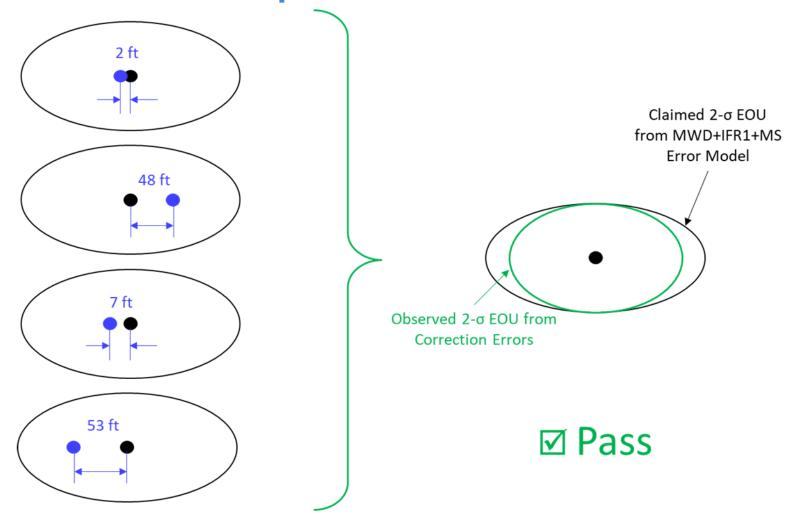
\*Use Chi-Squared distribution to determine pass/fail threshold for horizontal EOU
