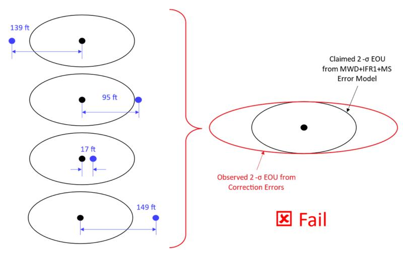
\*Use Chi-Squared distribution to determine pass/fail threshold for horizontal EOU
