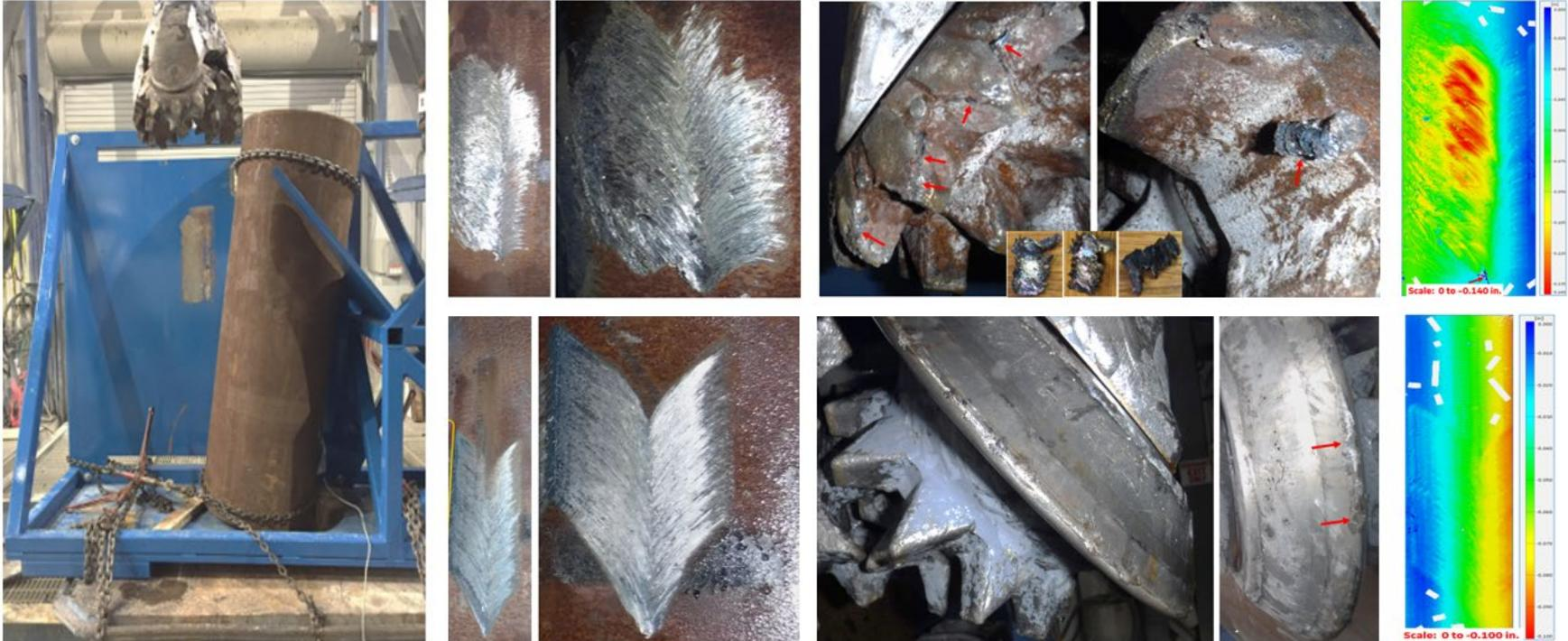
Laboratory Side Load Test Results – Casing Inclination 9°
