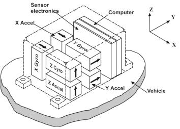
An IMU is an Inertial Measurement Unit – outputs raw rate and acceleration
