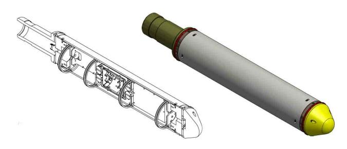
The concept was a core tube assembly containing all components, battery powered for 16 hours continuous operations with data logging for multiple operations. Housing was manufactured from DOM 4340. The end caps, nose cone and fishing neck were manufactured from 4340 bar stock.
