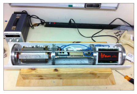
The core of W-PINS contains an IMU compartment, an IMU signal processing PCB and a processor, battery, storage compartment.
