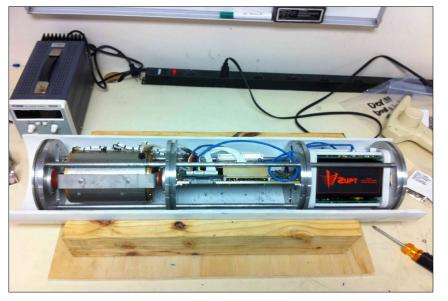
The core of W-PINS contains an IMU compartment, an IMU signal processing PCB and a processor, battery, storage compartment.
