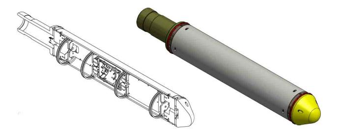
The concept was a core tube assembly containing all components, battery powered for 16 hours continuous operations with data logging for multiple operations. Housing was manufactured from DOM 4340. The end caps, nose cone and fishing neck were manufactured from 4340 bar stock.
