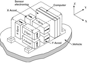
An IMU is an Inertial Measurement Unit – outputs raw rate and acceleration An INS is an Inertial Navigation System – outputs position, attitude, velocity An INS is an IMU with more signal conditioning and processing
