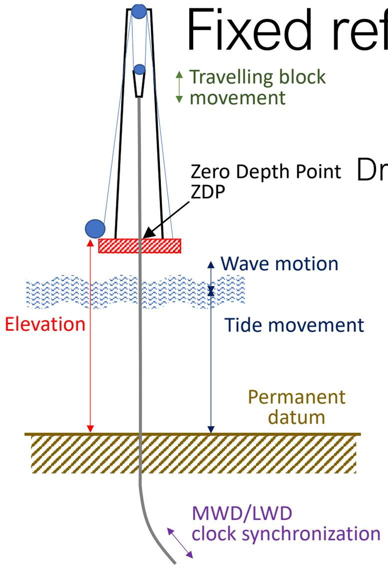
Drill pipe measurement reference point locational position and stability uncertainty
