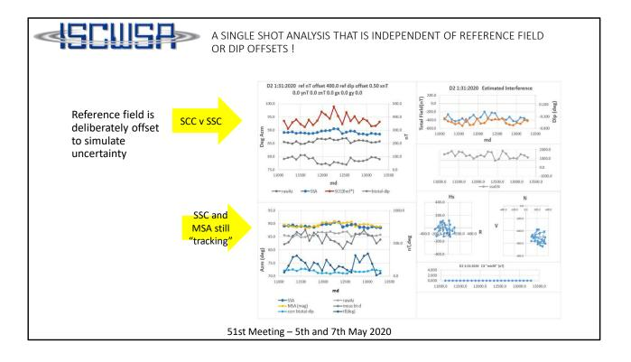
TO DEMONSTRATE THAT SURVEYS THAT ARE CORRECTED BY THIS METHOD ARE NOT SIGNIFICANTLY AFFECTED BY GEOMAGNETIC ACTIVITY OR REFERENCE FIELD OFFSETS OTHER THAN DECLINATION UNCERTAINTY, WE USED A DELIBERATELY INACCURATE REFERENCE FIELD. (POINT TO COMPARISON (POINT TO SSC AND MSA "TRACKING")
