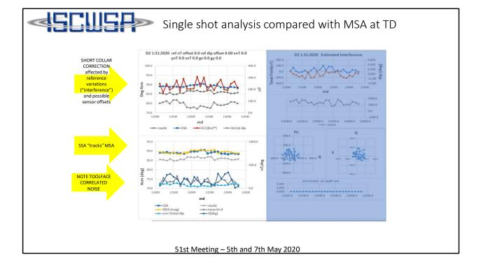
LOOKING MORE CLOSELY AT THE OVERALL RESULTS FOR THIS SECTION, **(POINT TO SHORT COLLAR RESULTS)** CLEARLY THE CONVENTIONAL SHORT COLLAR CORRECTION WE ARE USING HERE INTRODUCES SURVEY UNCERTAINTY FOR THE RAW SURVEY DATA AND REFERENCE FIELD VALUES AS PROVIDED BY INNOVA.
