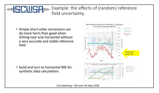
THIS SYNTHETIC EXAMPLE SHOWS HOW A DIURNAL OR MODERATELY ACTIVE REFERENCE FIELD CHANGES AFFECT CONVENTIONAL SINGLE SHOT DSI CORRECTIONS FOR A SIMPLE WELLBORE.
