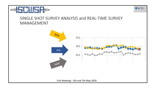
THESE MWD SURVEYS WERE CORRECTED ONE BY ONE FOR DRILLSTRING INTERFERENCE AND COMPARED WITH AN END-OF-JOB MSA ANALYSIS WITH THE HELP OF DATA AND MSA PROVIDED BY INNOVA LLC.
