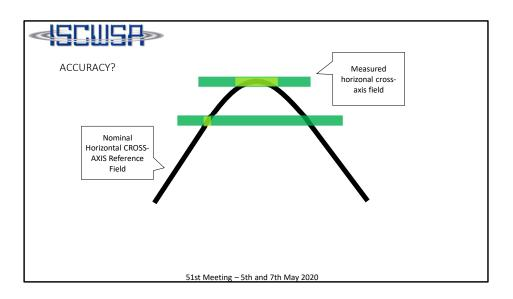
THE METHOD DOES NOT CORRECT FOR "LARGE" VARIATIONS IN THE REFERENCE FIELD OR INTERFERENCE FROM OFFSET WELLBORE CASING. THIS IS A SUBJECT FOR DISCUSSION, BUT NO TIME HERE. WE ARE TRYING TO STAY WITH A "SIMPLE" SINGLE SHOT METHOD. HOWEVER, AS NEEDED, IT WOULD BE POSSIBLE TO "UPDATE" THE REFERENCE FIELD ESTIMATES AFTER SEVERAL QUIET SHOTS.
