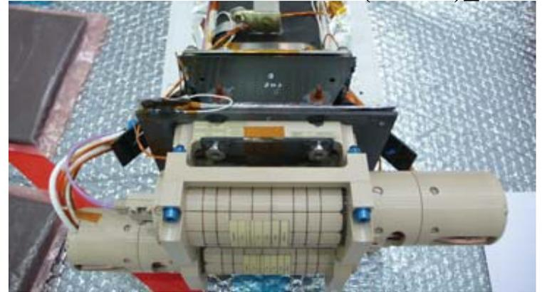
Optical bench: vector field magnetometer and 3-head star camera (Denmark)
