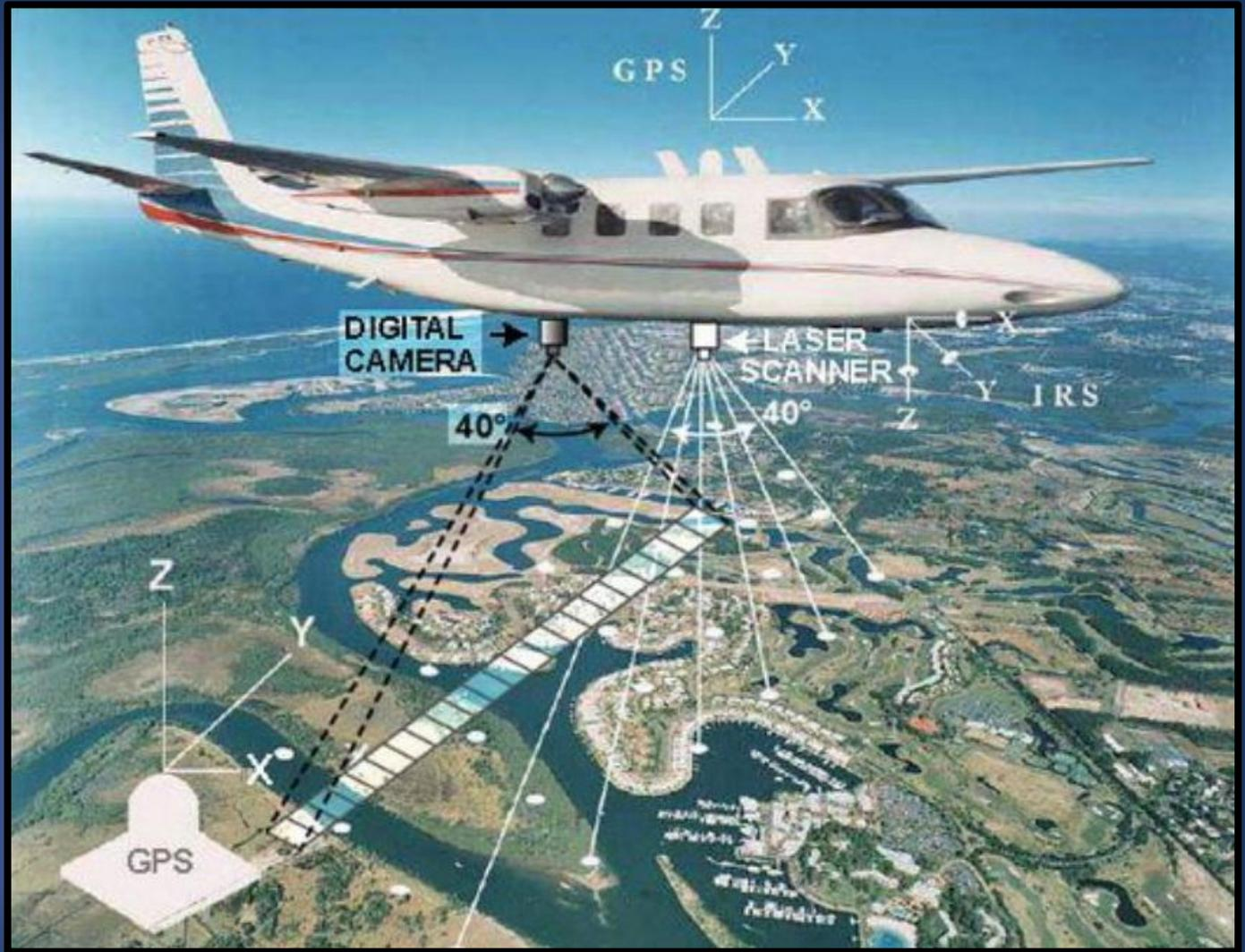
**LiDAR mapping from aircraft**
