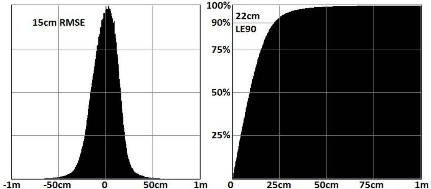
**Elevation differences between the PhotoSat WV3 and LiDAR topography.**
