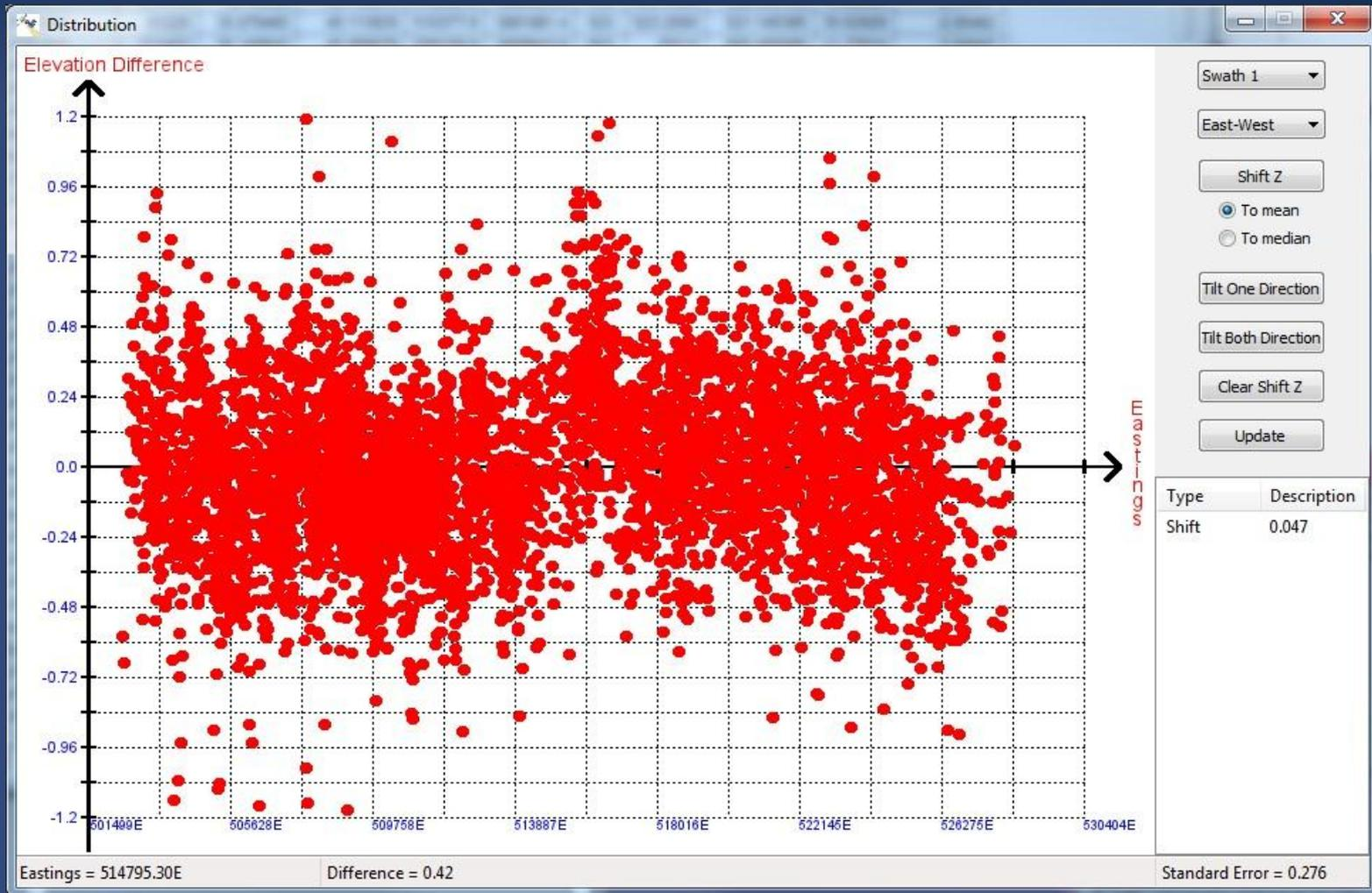
**Kurdistan seismic source points differences to satellite elevations, SE points raised 1.3m
