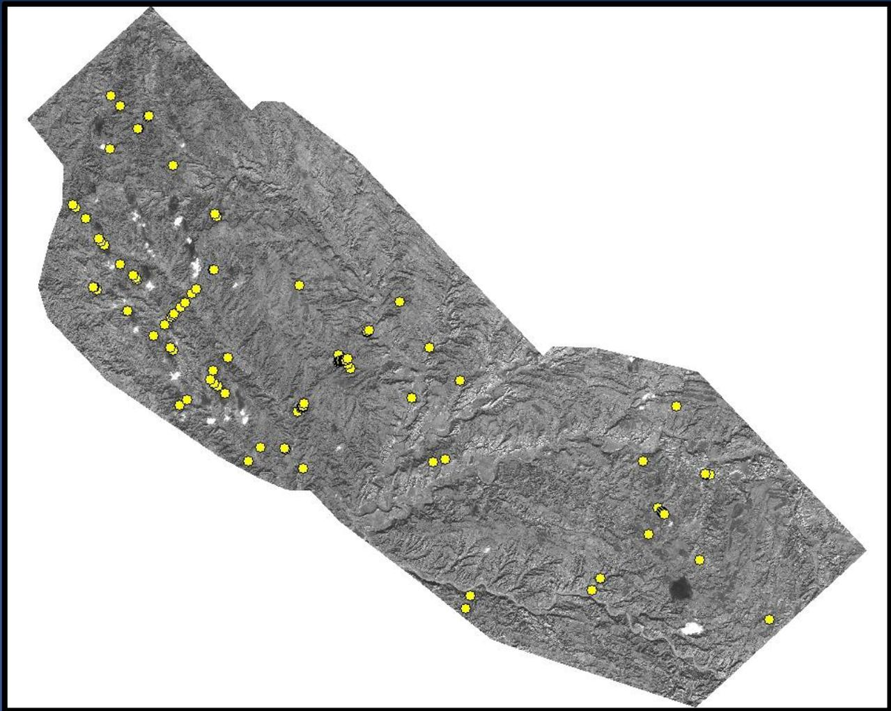
**107 seismic source points with greater than 1m elevation difference to satellite elevations. These are probably survey errors due to too few GPS satellites in range. These source point elevations should be replaced by the stereo satellite elevations.**
