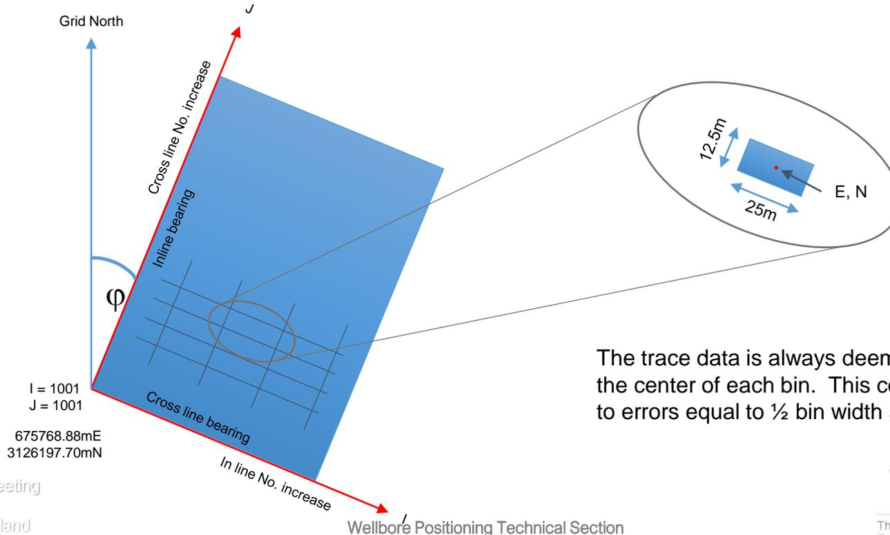
The trace data is always deemed to be deleted at the center of each bin. This could potentially lead to errors equal to  $\frac{1}{2}$  bin width along both axes.
