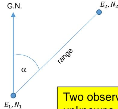
Two observations, two unknowns, no redundancy. Cannot detect gross errors.
