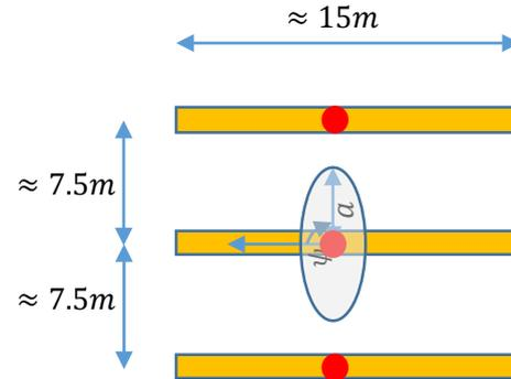
Error ellipse computed from  $C_{\hat{x}}$ , to determine semi major axis and orientation. Cross line precision will exceed in-line precision.
