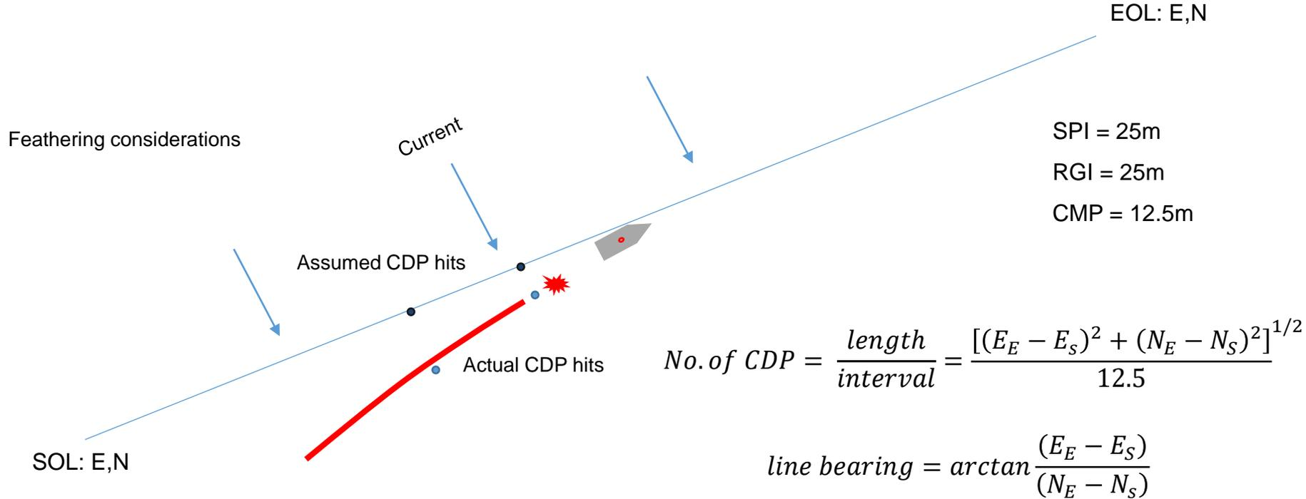
Trace positions interpolated between SOL and EOL at 12.5m intervals along a bearing computed using the SOL and EOL coordinates. Therefore, trace data is assumed to occur on the pre-plot line. This is very seldom the case. What effect on precision?
