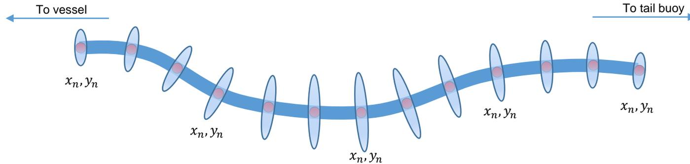
Error ellipses are initially derived from  $C_{\hat{x}}$  for acoustic nodes within the network, which enables the precision of each receiver group to be interpolated.
