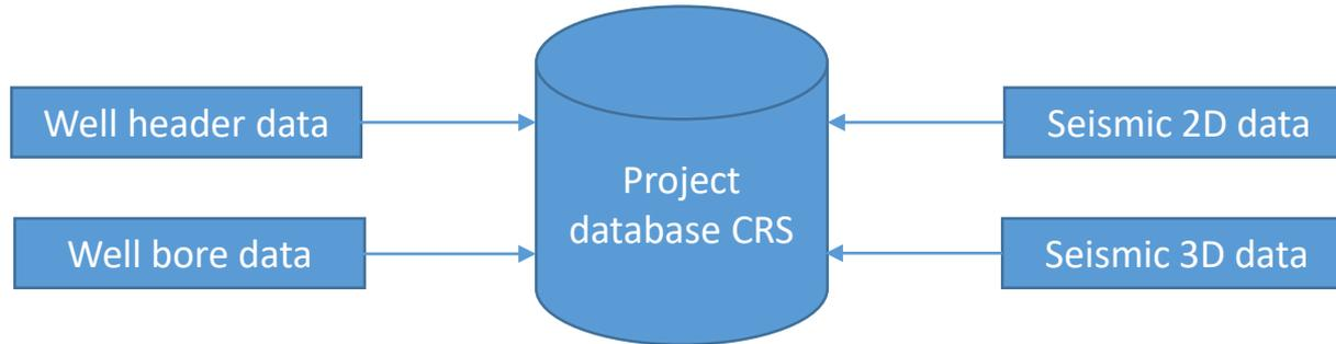
Maintaining integrity requires data loaders select the correct parameters for the data. Most importantly selecting the CRS associated with the data. Incorrect choice may introduce horizontal error with a magnitude of many hundreds of meters. This will have a direct impact on the proposed well header coordinates.
