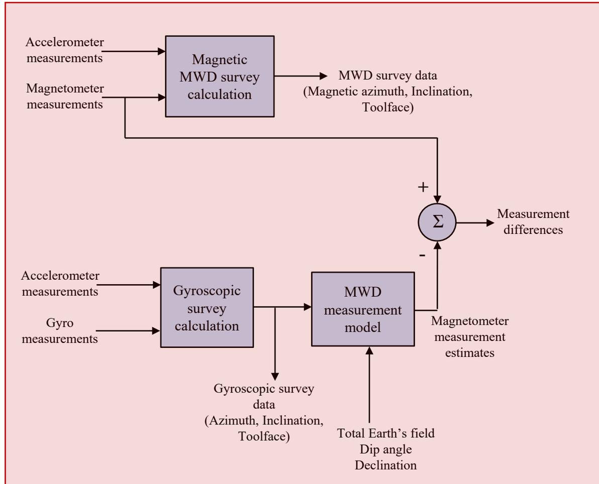
Estimates of the MWD magnetometer readings are generated based on:
