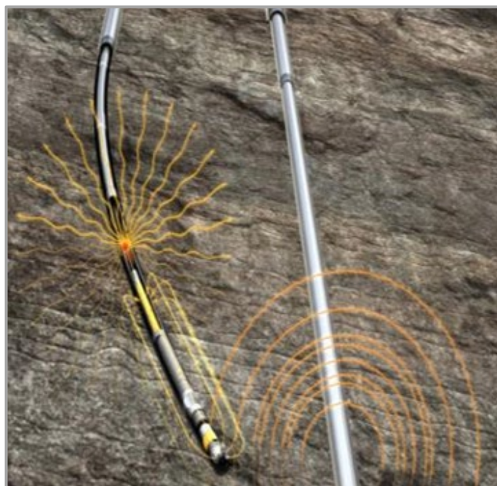
Figure 23—AI-AMR system diagram. No target well access. A wireline conveyed AMR tool injects the formation with AC current creating an induced magnetic field in the target well casing.
