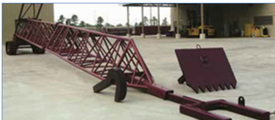
Figure 123—Rakes (right), are metal devices that may be attached to the end of the Athey Wagon to grab the debris and drag it away from the wellhead and surrounding area.
