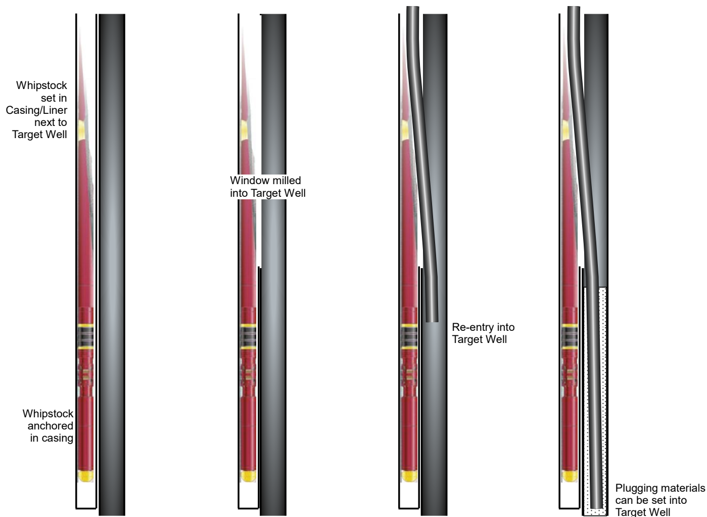
Figure 113—Cased hole whipstock milling method concept
