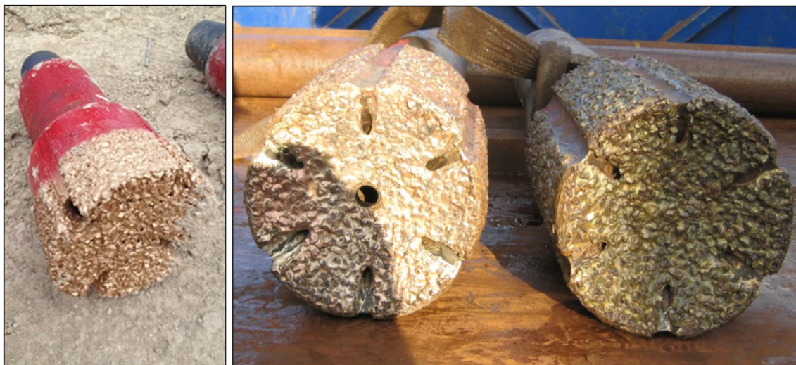
Figure 114—New Concave Face Mills. The orientation of the jets, the gauge lengths, and the total mill length are chosen based on targeted window length and actual incidence angle achieved at the point of contact. Then the milling parameters must be optimized to ensure effective milling performance. In most cases, multiple face mills are required when cutting through multiple concentric tubular strings.
