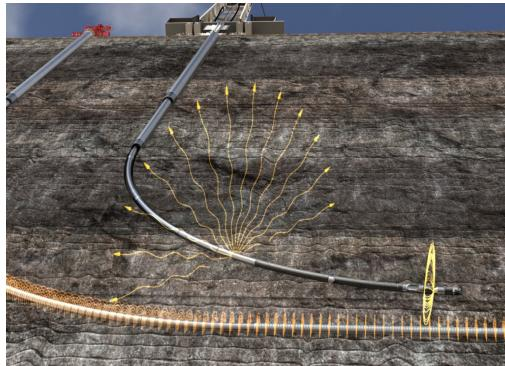
The magnetic field is analyzed, and a distance and direction to the target is calculated.
