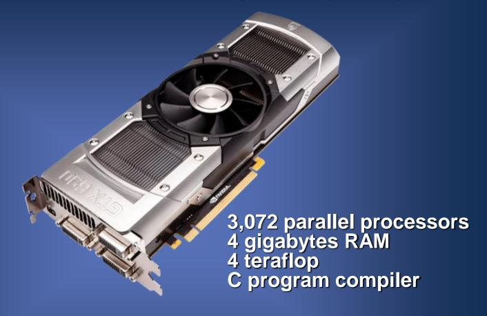
GPUs perform numerical processing up to 1000 times faster than CPUs. This enables us to do the hundreds of millions of 2D Fourier transforms necessary to automatically produce 1m Digital Surface Models from stereo satellite photos in reasonable times.
