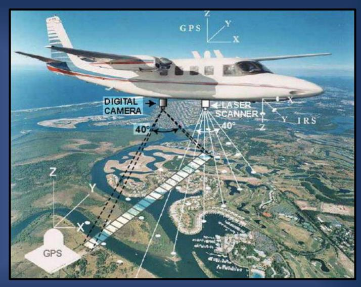
LiDAR mapping from aircraft
