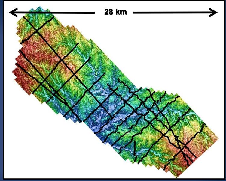
2D seismic source points
