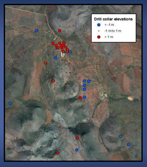
Drill hole collar elevation differences between the GPS survey and the stereo satellite mapping
