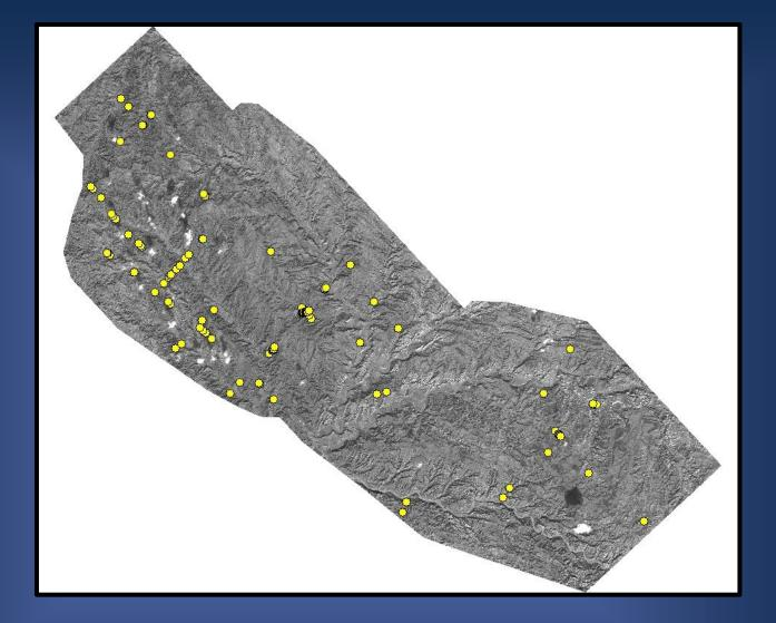
107 seismic source points with greater than 1m elevation difference to satellite elevations. These are probably survey errors due to too few GPS satellites in range. These source point elevations should be replaced by the stereo satellite elevations.
