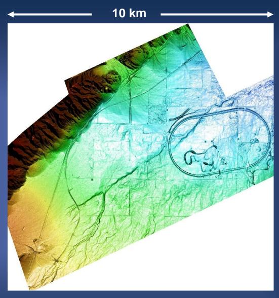
Open Topography LiDAR DTM. 5cm accuracy.
