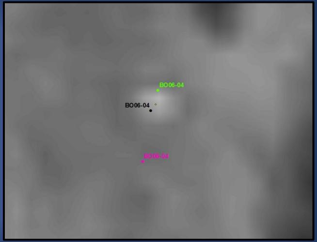
40cm x 40cm white concrete block on satellite photo and the coordinates from the three GPS surveys
