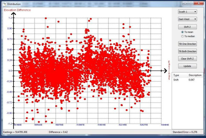
Kurdistan seismic source points differences to satellite elevations, SE points raised 1.3m Standard deviation 28cm.
