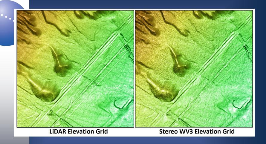
500m width CSH - Lidar vs PhotoSat
