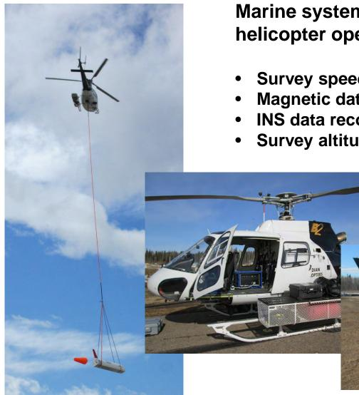
Marine system now modified for helicopter operation
