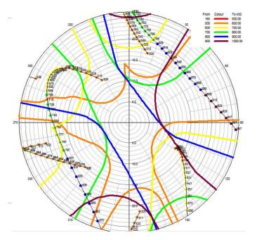
North referenced, normal plane travelling cylinder diagram
