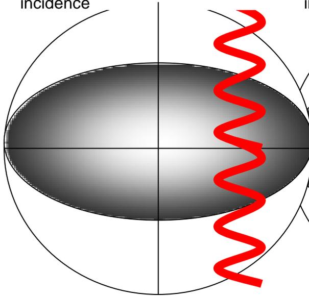
Traveling Cylinder Plot Showing Wellbore with tortuosity at 2 degree incidence
